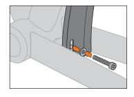
**ATTENTION! MOUNTING OF SPACERS FOR FRAMES WITH DISC BRAKES**
