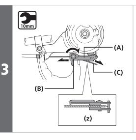
Pull the link (A) back until it stops. Then, while pulling the inner cable (C) to apply the full amount of tension to the cable, tighten the inner cable fixing nut (B).
