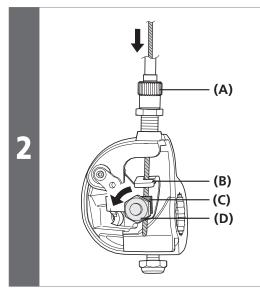
Fit the inner cable into the link **(B)** in the bell crank.
