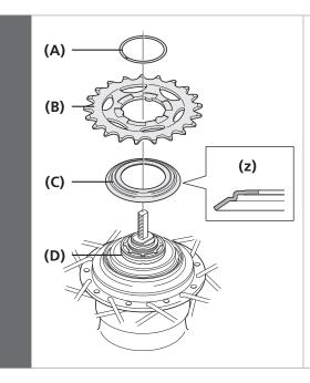
Place the right-hand waterproof cap C (C) onto the driver (D) on the right side of the hub body.
