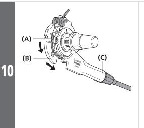
Mount the inner cable (A) to the pulley (B) as shown in the illustration.
