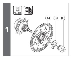
Install the disc brake rotor (A) to the hub.
