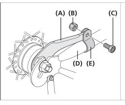
Install the brake arm (A) to the chainstay (D) using the arm clip (E) and temporarily tighten the clip bolt (C) and clip nut (B) loosely.
