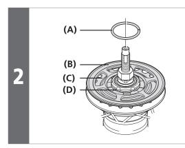
Install the CS-S500 sprocket (C) to the driver (D) on the right side of the hub body with the guard plate (B) facing outward, and secure it in place with the snap ring (A).
