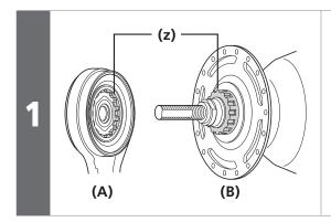
Engage the splines on the hub body (B) with the splines on the inter-M brake (A), and then provisionally tighten the brake unit fixing nut.
