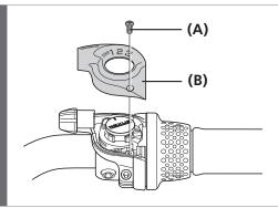
Loosen the cover fixing screw (A), and then remove the indicator cover (B).
