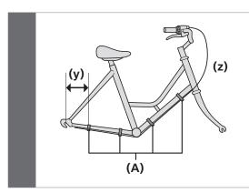
Secure the cable to the frame with the outer casing bands (A).
