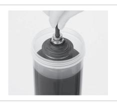
Keep the internal unit immersed for approximately 90 seconds.
