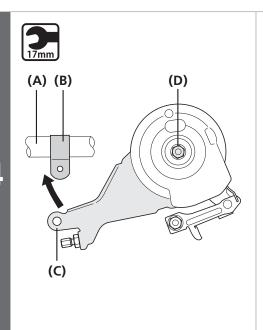
Install the brake arm **(C)** of the inter-M brake to the chainstay **(A)** using the arm clip **(B)** and temporarily tighten the clip bolt and clip nut loosely.
