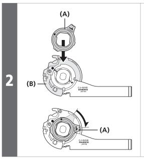
Secure the cassette joint to the hub with the cassette joint mounting ring (A).
