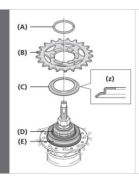
Place the right-hand waterproof cap B **(C)** onto the driver **(D)** on the right side of the hub body.
