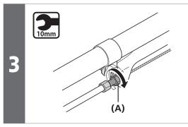
After depressing the brake lever to check the braking performance, secure the cable adjustment barrel with the cable adjusting nut (A). (A) Cable adjusting nut
