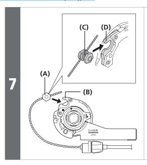
Bring the cable around to the cassette joint pulley (B), hold it so that the inner cable mounting nut (A) is facing outwards (towards the dropout), and then slide the flats part (C) of the inner cable mounting washer into the gap (D) in the pulley.
