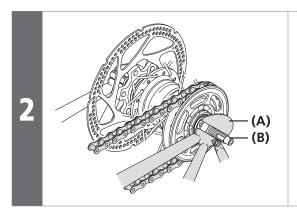
Mount the chain on the sprocket, and then set the hub axle (B) into the dropout (A).
