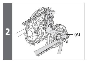
Mount the chain on the sprocket, and then set the hub axle into the dropout.
