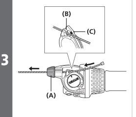
Set the inner cable onto the pulley.
