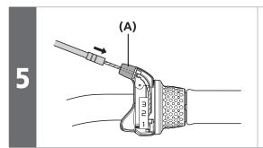
Insert the outer casing into the outer casing holder (A).
