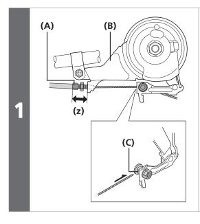
Place the cable adjustment barrel (A) so that it is 15 – 17 mm from the end of the brake arm (B), and then pass the inner cable through the cable adjustment barrel of the brake arm and then through the hole in the inner cable fixing bolt (C).
