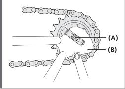
Mount the chain on the sprocket, and then set the hub axle (A) into the dropout (B).
