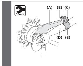
Fix the brake arm (A) securely to the chainstay (D) with the arm clip (E).
