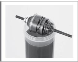
After lubrication is complete, reassemble the hub.
