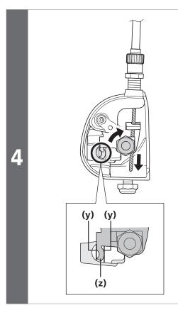
With the inner cable kept tight, tighten the inner cable mounting nut while positioning the end of the link between the two white lines on the window.
