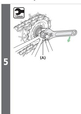
Take up the slack in the chain and secure the wheel to the frame with the flange nut (A). (A) Flange nut
