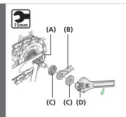
If the total width of the dropout and other parts such the stand and mudguard stay (B), on the right side of the hub axle, is 8.5 to 11.5 mm
