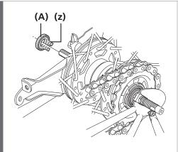
Place the non-turn washer **(A)** onto the left side of the hub axle from the outer side.
