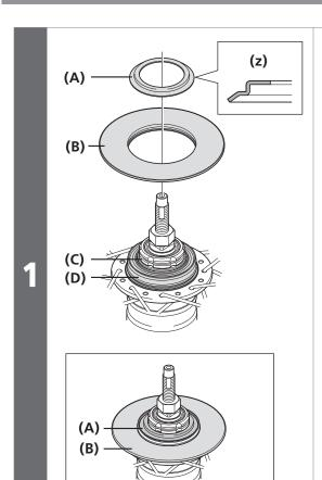
Install the chain guard (B) to the right-hand waterproof cap A (D) of the hub body, and then install the right-hand waterproof cap B (A) to the driver
