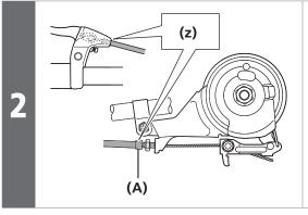
Check that both ends of the outer casing are securely inserted into the cable adjustment barrels (A) of both the brake lever and brake arm.
