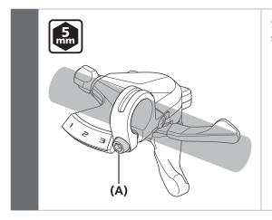
Secure the shifting lever using the clamp screw (A).
