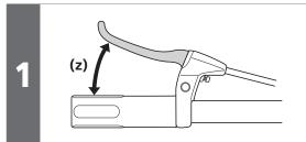
After checking that the wheel does not easily turn while the brake cable is being pulled, depress the brake lever about 10 times as far as the grip in order to run in the brake cable.
