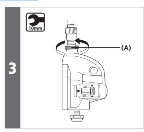
After adjusting the bell crank IV, fix the cable adjustment barrel with the cable adjustment nut (A).
