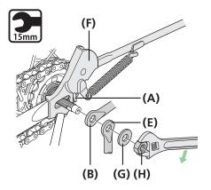
If the total width of the dropout and other parts such the stand **(F)** and mudguard stay, on the right side of the hub axle, is 14.5 to 17 mm
