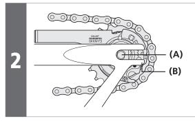
Mount the chain on the sprocket, and then set the hub axle (A) into the dropout (B).
