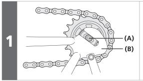
Mount the chain on the sprocket, and then set the hub axle (A) into the dropout (B).
