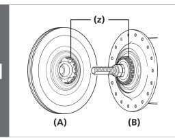
Engage the splines on the hub body (B) with the splines on the inter-M brake (A), and then provisionally tighten the brake unit fixing nut.
