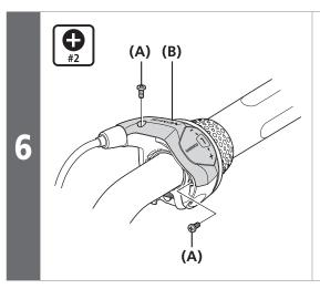
Fasten the cover **(B)** with the 2 cover fixing screws **(A)**.
