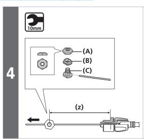
After checking that the end of the outer casing is pushed all the way to the back of the outer casing holder of the shifting lever, insert the inner cable into the inner cable mounting bolt (C).
