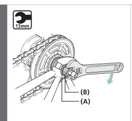
Take up the slack in the chain and secure the wheel to the frame, using a 3.2 mm washer (A) and a 9 mm hub nut (B) on the right side and a cap nut on the left side of the hub axle.
