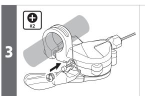
Pass the inner cable through and install the inner hole cap.
