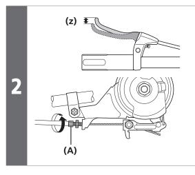
Turn the cable adjustment barrel (A) so that there is about 15 mm of gap (z) in the brake lever.
