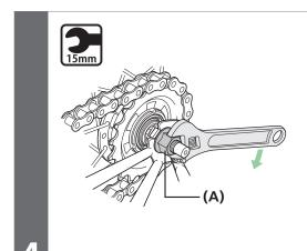
Take up the slack in the chain and secure the wheel to the frame with the flange nut (A). (A) Flange nut
