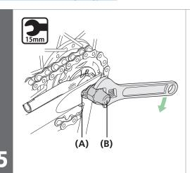
Take up the slack in the chain and secure the wheel to the frame with the cap nut (B).
