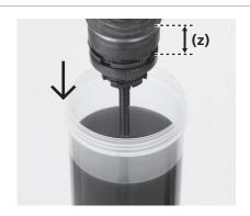
Immerse the internal unit into the oil from the left side until the oil reaches up to ring gear unit 1, as shown in the illustration.
