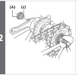
Place the non-turn washer **(A)** onto the left side of the hub axle from the outer side.
