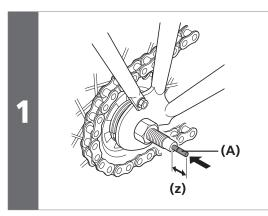
Insert the push rod (A) into the hub axle.
