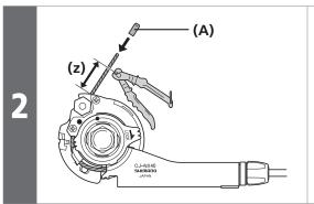
After adjusting the cassette joint, cut off the excess length of inner cable. Then install the inner end cap (A).
