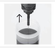
Remove the internal unit from the oil.
