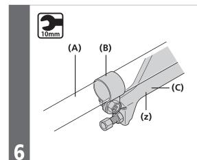
Fix the brake arm **(C)** of the inter-M brake securely to the chainstay **(A)** with the arm clip **(B)**.
