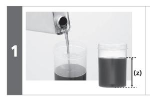
Fill the bottle with maintenance oil to a height of 95 mm.
