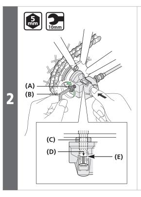
While pushing the bell crank into the hub axle, align the splines inside the bell crank with the hub nut (C), and continue push until the crank comes into contact with the end face (E) of the hub axle.
