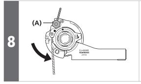
Turn the cable  $60^{\circ}$  counterclockwise and attach it to the hook **(A)**.
