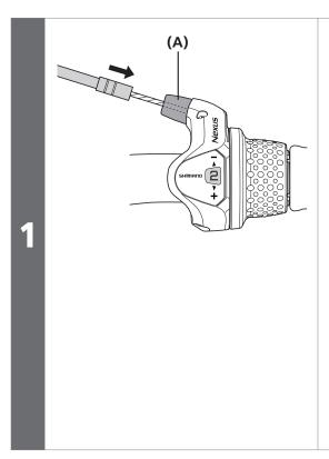
Insert the outer casing into the outer casing holder (A).
