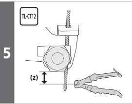
After tightening the inner cable mounting nut, cut off the excess length of inner cable.
