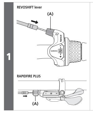
Insert the outer casing into the outer casing holder (A).
