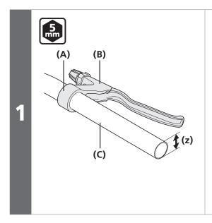
Install the brake lever (B).
