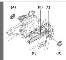
Place the non-turn washers (A) and (D) onto the right and left side of the hub axle.
