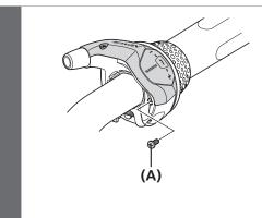
Loosen the two cover fixing screws (A) and remove the cover (B).
