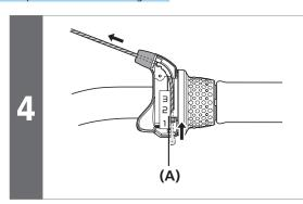
Pull the inner cable so that the inner cable drum fits into the recess in the winder unit (A).
