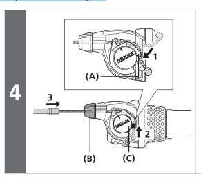
Hook the inner cable into groove in the pulley **(A)**, and pull the inner cable so that the inner cable drum fits into the hole in the pulley **(C)**.
