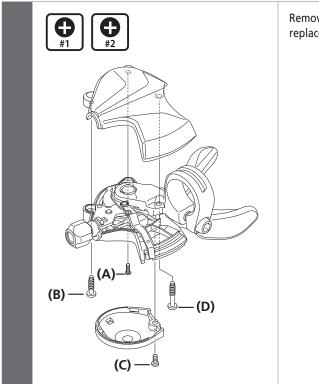
Remove the four mounting screws, and replace the cover.
