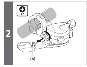
Remove the inner hole cap (A).
