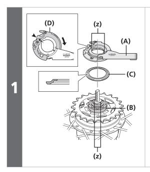
Install the driver cap **(C)** to the driver **(B)** on the right side of the hub body.
