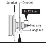
Total width of the dropout and other parts such the stand and mudguard stay: 4 to 7.5 mm (Axle length: 168 mm / 175 mm)
